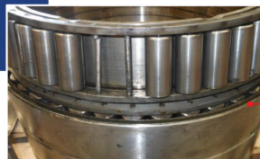
Premature failure of low quality no-brand cage-roller assembly F-802030.TR4/LM274449DW.410.410D
