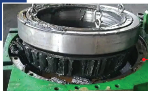
Catastrophic failure of low quality no-brand pierced roller bearing M 274149 DW/110!!!
