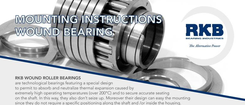
Although before being mounted the spiral inner ring diameter is smaller than the mating shaft diameter and the spiral outer ring diameter is larger than the housing hole diameter, on the other hand once properly installed both the rings have to result in interference fit. By the light of this prescrition it is recomended a final check at the end of the mounting to be sure to get a roper interference fit on both bearing rings.
