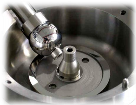
Fig. 6 – Ball-on-washer life prediction testing rig
