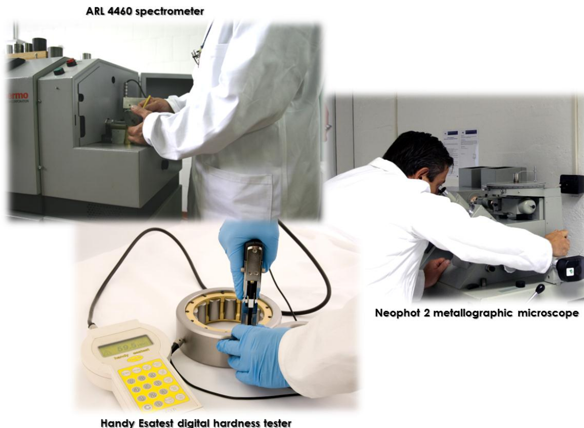
Fig. 23 – Metallographic and mechanical measuring equipment
