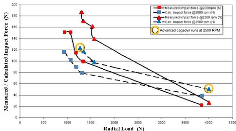
Fig. 15 – Measured and calculated roller-cage impact forces
