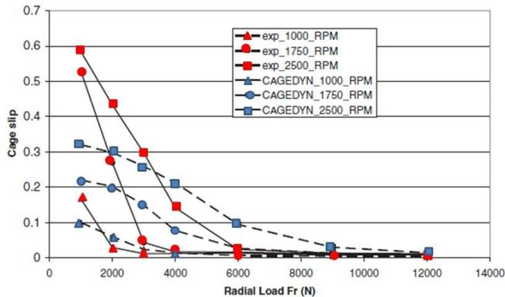
Fig. 9 – Calculated and measured cage slip for inch size tapered roller bearing 74000
