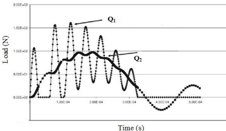
Fig. 12 – Hertzian load  $Q_1$  and bridge load  $Q_2$
