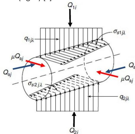
Fig. 6 – Roller skewing in misaligned cylindrical roller bearing
