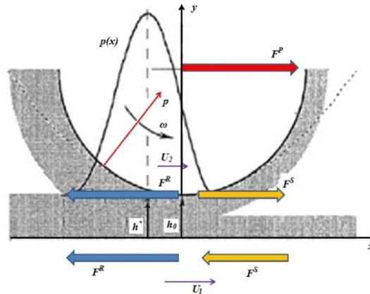
Fig. 14 – Description of the hydrodynamic rolling and pressure force and sliding force
