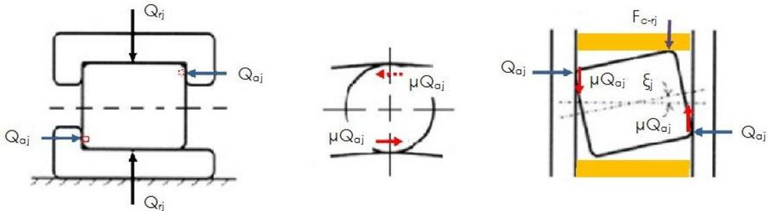
Fig. 7 – Roller skewing in cylindrical roller bearing
