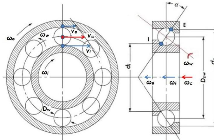
Fig. 5 – Simple kinematics for moderate speed conditions
