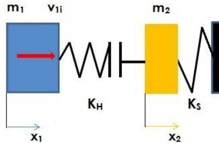
Fig. 11 – Model of the roller-cage impact dynamic simulation
