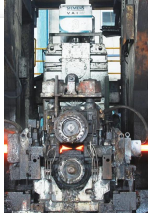
SIEMENS VAI horizontal stand for S240, S340, S400 and S500 rebar from 5,5 to 28 mm diameter (Malaysia)
