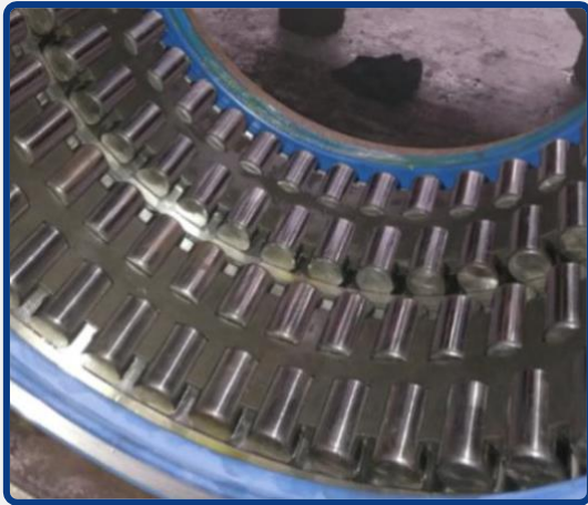
RKB R 635194 mounted on SMS Meer stand (Germany) with grease lubrication
