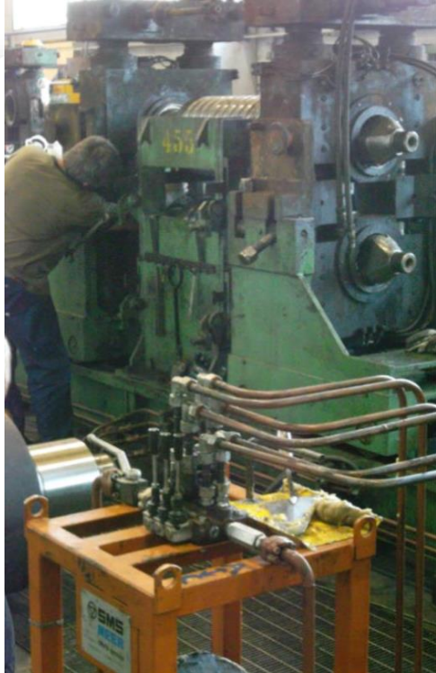
SMS MEER horizontal stand for rebar from 9,5 to 19,1 mm diameter (France)
