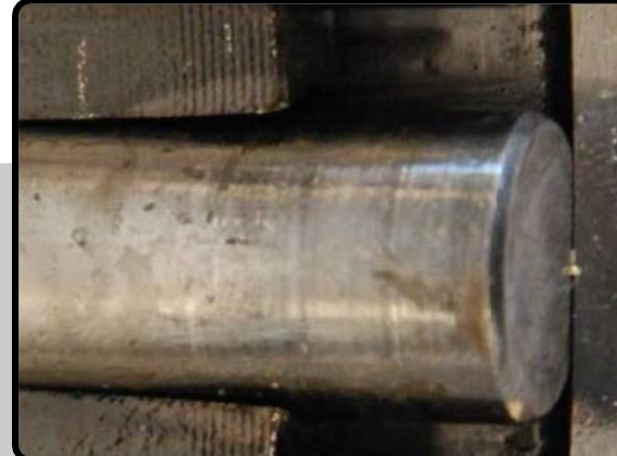
Cage tenon damage!
