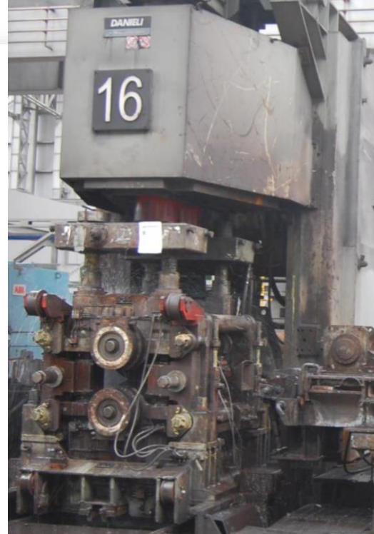
DANIEMI horizontal stand for corrugated steel bars (grade 42) production (Italy)
