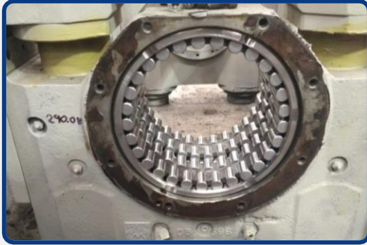
RKB R 313811 mounted on Danieli stand (Mexico) with oil mist lubrication
