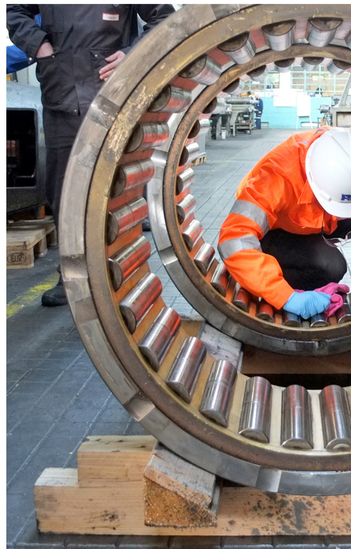
Rkb multiroll bearing for aluminum rolling mill, optimized for air-oil lubrication and automatic roll changing device.
